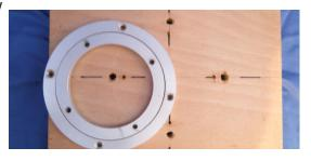
Unscrew the turntable and clamp your two pieces of wood together, carefully aligned. Using the small holes in the base as a guide, drill into the top piece, not all the way
